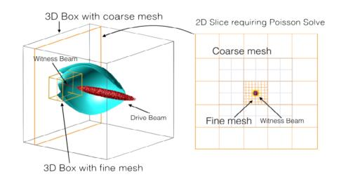
Interpolate field on coarse grid  $\phi_l$  onto the boundary of  $\phi_{l+1}$  Use FFT solver to solve  $\phi_1$ , multigrid algorithm to solve  $\phi_{l>1}$
