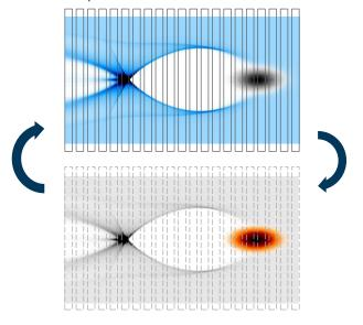
**3D loop**: field and plasma particles are frozen while beam is advanced.
