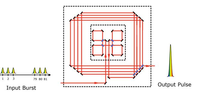
A 4+4 multiplexed GTI system temporally combines 81 pulses into 1 output pulse
