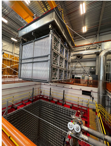
Detector extracted from ATF, rotate and inserted inside the cryostat
