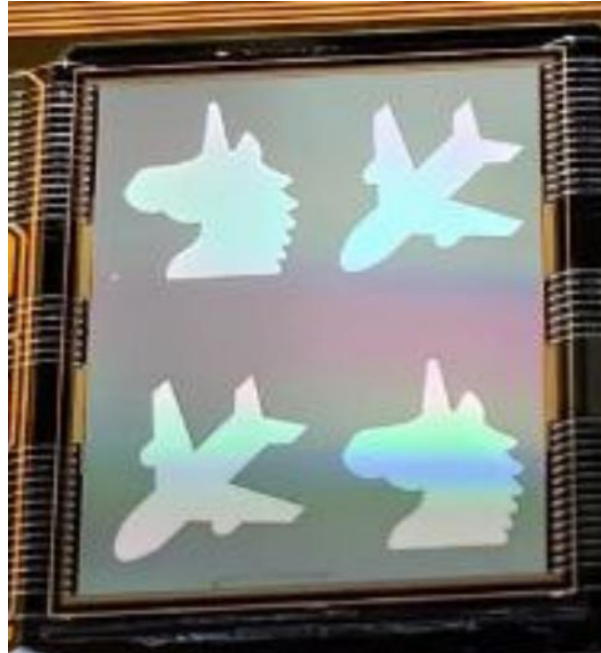
Aluminum shield to blind visible and IR photons*
