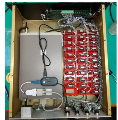
Internal view of the newly developed MUX
