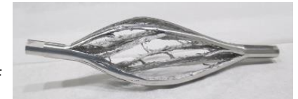
Thermal shock effect in an Iridium rod exposed to a high-intensity beam pulse at CERN's HiRadMat facility
