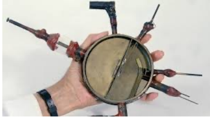
Ernst Lawrence's first cyclotron, 1929 (Berkeley). Proton energy: \sim 1 MeV
