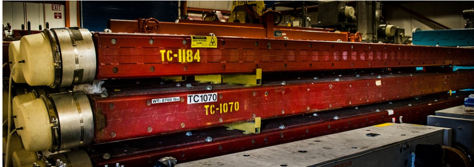
Superconducting magnets for the Tevatron, first industrial scale use of such magnets
