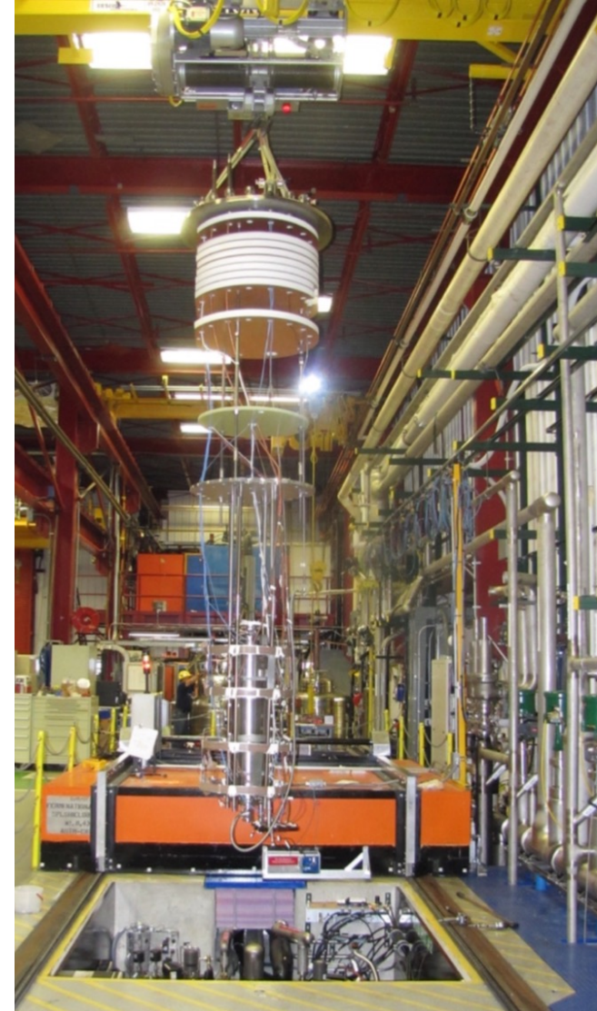
Fermilab Vertical Test Stand used for liquid helium tests of accelerator SRF cavities
