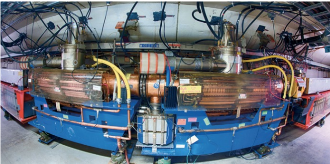
Booster 8 GeV Rapid-cycling synchrotron 0.5 km circumference
