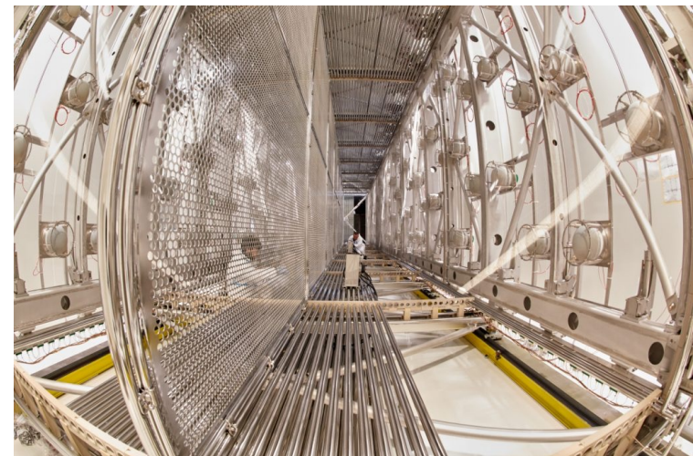
View of one of the ICARUS detector's inner time projection chamber (TPC): Cathode plane on the left, wire plane and PMT array on the right
