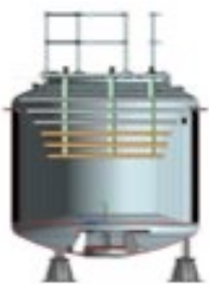
COLOSSUS - creating the world's largest dilution refrigerator, operating at millikelvin degrees
