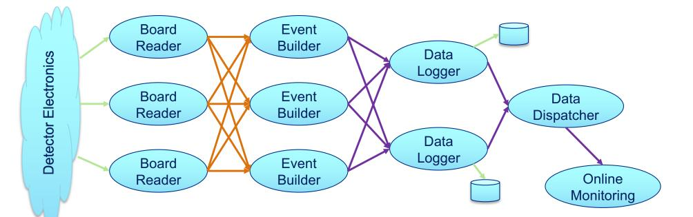
Initial contents are raw data from electronics (plus artdaq-added header)
