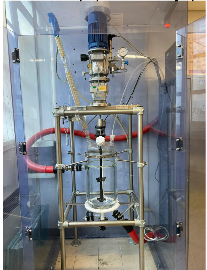
The reactor to prepare the MMA syrup
