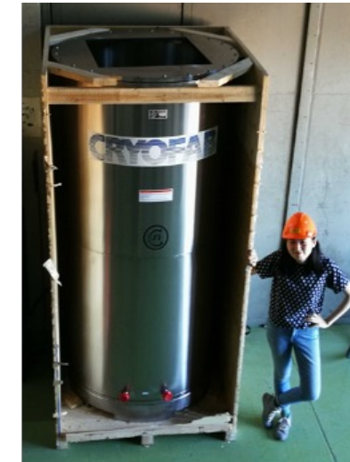
Single Module Cryostat
