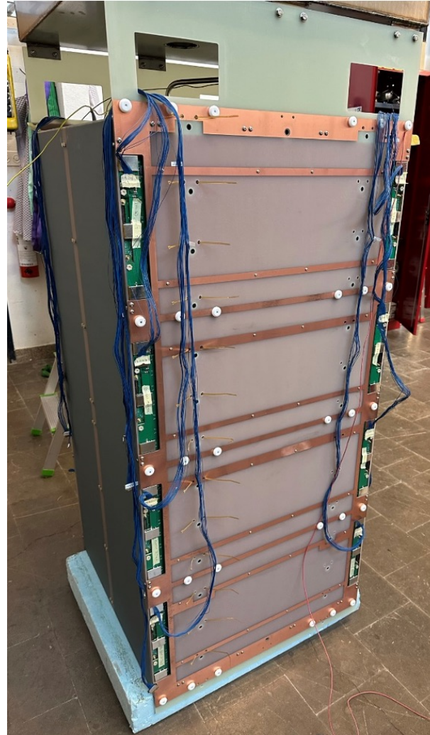
Example: LArPix-v2b system, 102,400 pixels, 3.8mm spacing
