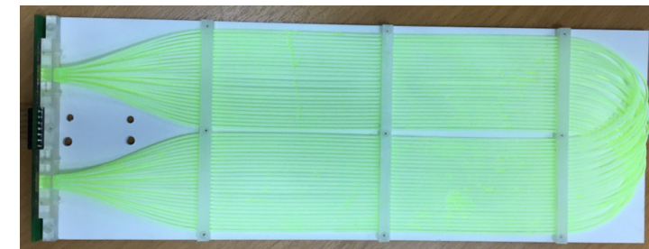
Fiber-bundle style light trap: JINR LCMs
