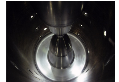
Region between the inner and outer conductors.
