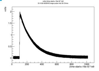
Start w/ measured sipm response, large LASER pulse, no amplifier
