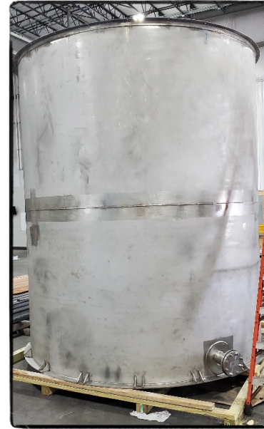
EOS outer steel and inner acrylic tanks
