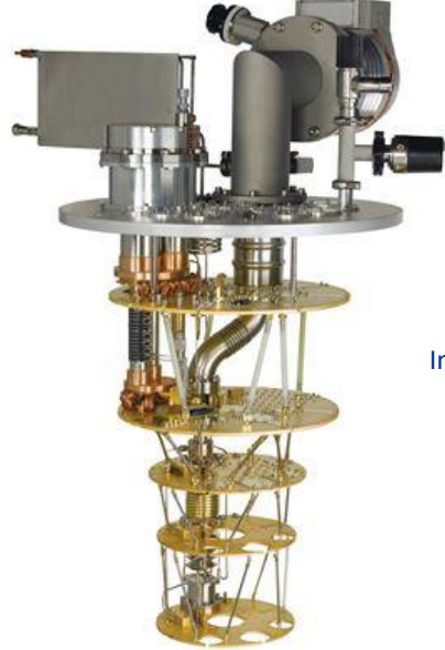
Standard fridges Mixing chamber diameter ~300mm Minimum temperature ~10 mK
