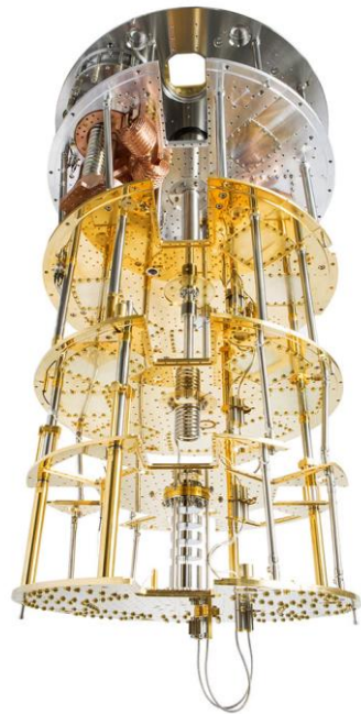
Large frame fridges Mixing chamber diameter ~500mm Minimum temperature ~10 mK
