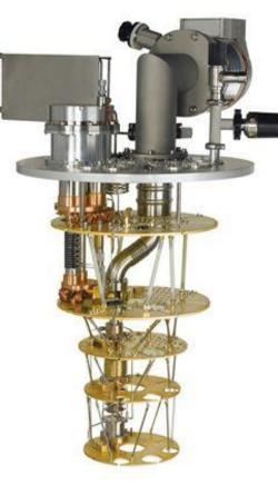
Standard fridges Mixing chamber diameter ~300mm Minimum temperature ~10 mK
