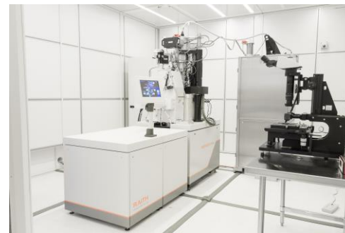
Raith EBP5200 E-Beam lithography system (100 kV)
