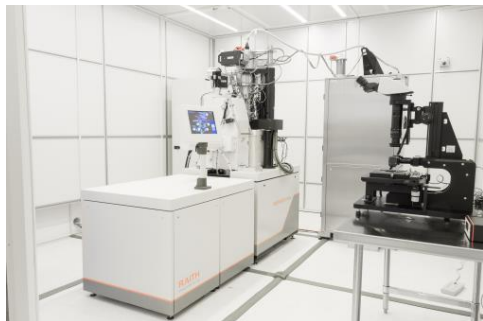
Raith EBP5200 E-Beam lithography system (100 kV)
