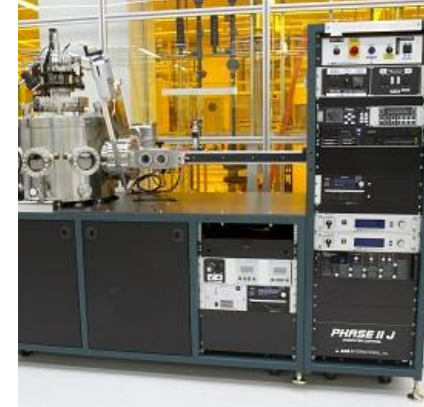
AJA ATC 2200 UHV Sputtering System
