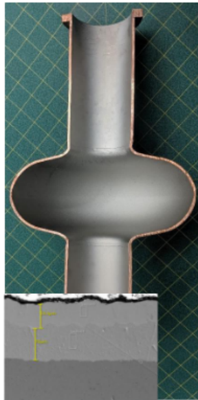
CVD Nb 3 Sn coating on CVD niobium interlayer on welded (Niowave) copper cavity substrate
