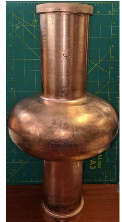
SN-4A, seamless copper cavity substrate (BTM, Inc.)
