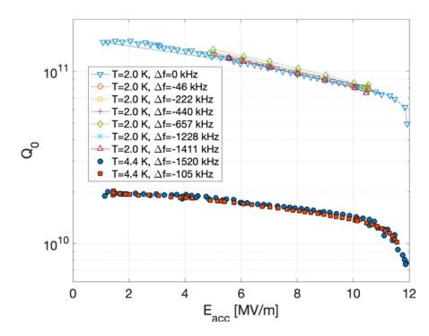
Strong degradation in the coated cavity performance after room temperature tuning for 200 kHz
