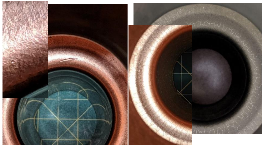
Left , SN-2, as-received surface roughness and anomalies; right , SN-4, post-etch copper and as-coated & as-tested.
