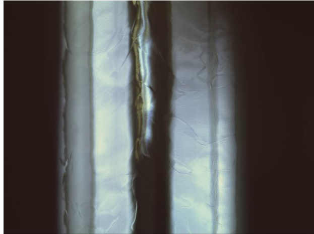
Example of iris grinding on 3-cell cavity Picture courtesy of H. Araki
