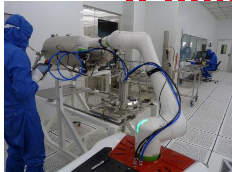
Operator programming the pathway of the effector to the coupler flange of the cavity while the coupler is prealigned
