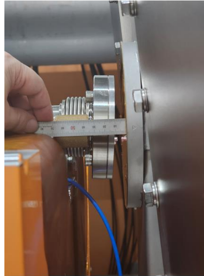
10 mm between assembly parts, working area less than 10 cm
