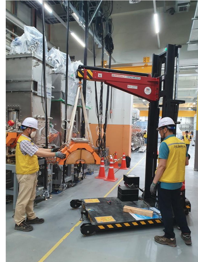
Movable crane for lifting the top side of quadrupole magnet
