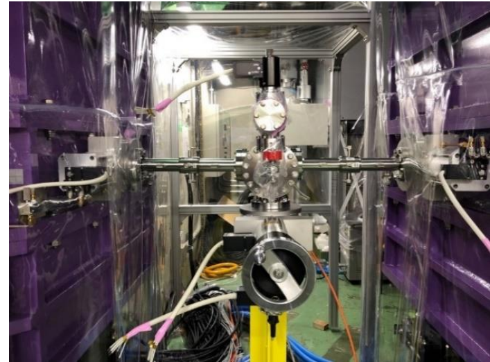
Mounting of upper half of Q-mag.
