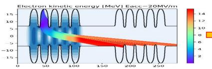
**Single emitter** trajectories calculation with <u>one cavity powered</u> (CAV4) while the adjacent is off (CAV3). Trajectory colours are determined with respect to the electrons kinetic energy. All the impact on the beam tubes and adjacent cavity have energies between 12 and 15MeV.
