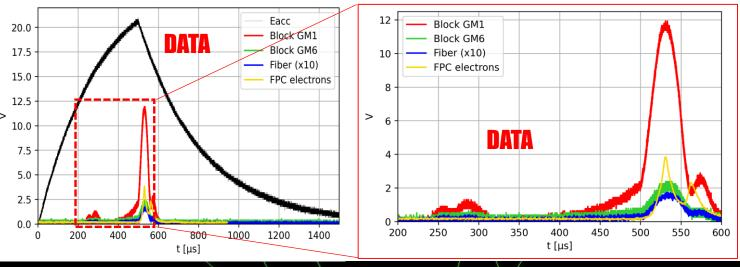
CAV4 excited with **500µs square pulse**, the maximum Eacc is about 20MV/m (black). It is possible to appreciate the **electron current detected by the pick up in the fundamental power coupler** (**gold**) and the radiation detected by the plastic scintillator at the cryomodule ends, block at GM1 position (red) block at GM6 position (green) and fiber (blue).
