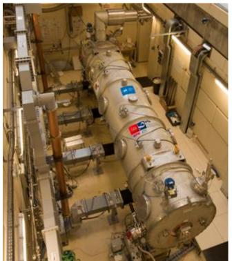
ESS cryomodule installed in the test stand at Saclay
