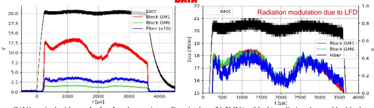
CAV1 excited with **nominal pulse**, the maximum Eacc is about <u>21.2MV/m</u> (black), radiation detected by block at GM1 position, close to cavity (red), radiation detected by block (green) and from fiber (blue). *Right: zoomed and normalized view of the same pulse where it is possible to appreciate closely the change in the radiation amplitude due to Lorentz force detuning.*
