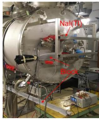
Scintillator block installed on ESS cryomodule during power test in Saclay, close to a NaI(Tl) scintillator.
