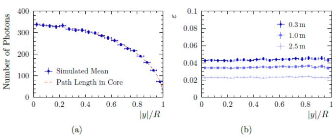
Figure 3.36: Dependencies of mean number of produced photons per MIP (a) and ratio of photons reaching one fibre end  $\varepsilon$  (b) on distance |y| of the MIP's trajectory from fibre axis. The dashed line in (a) shows a trend proportional to the MIP's path length in the fibre core. Values in (b) are obtained at three distances x of the excitation from the fibre end.
