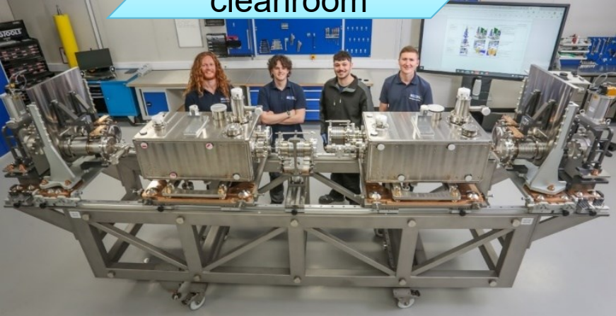
Cavity string pre-cleanroom
