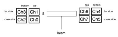
Four 6mmx6mm SiPMs on each side 0-3 on the S side 4-7 on the E side
