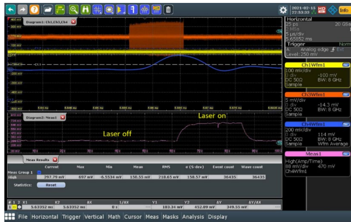
Figure 1-52. With the laser off the background was measured to be 2 nA at the Faraday Cup. When the laser was on the signal went to 600 mV which corresponded to 6 nA at the Faraday Cup.
