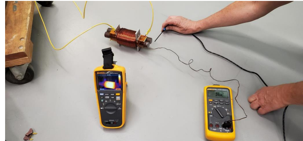
Thermal testing of magnet assembly for analysis correlation:
