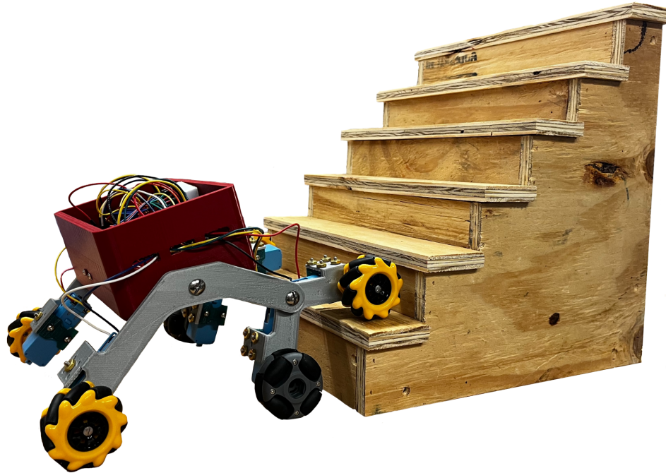
Figure 3. Scaled-down RD robot and stairs used for prototyping and testing.
