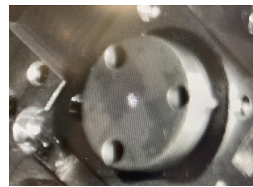
Nb 3 Sn sample. The sample was located close to the heater during the coating process.
