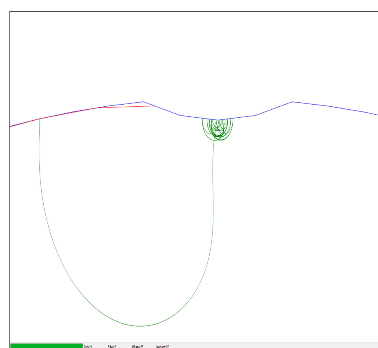
Figure 8: Multipaction of LB650 Cavity with Weld Bead
