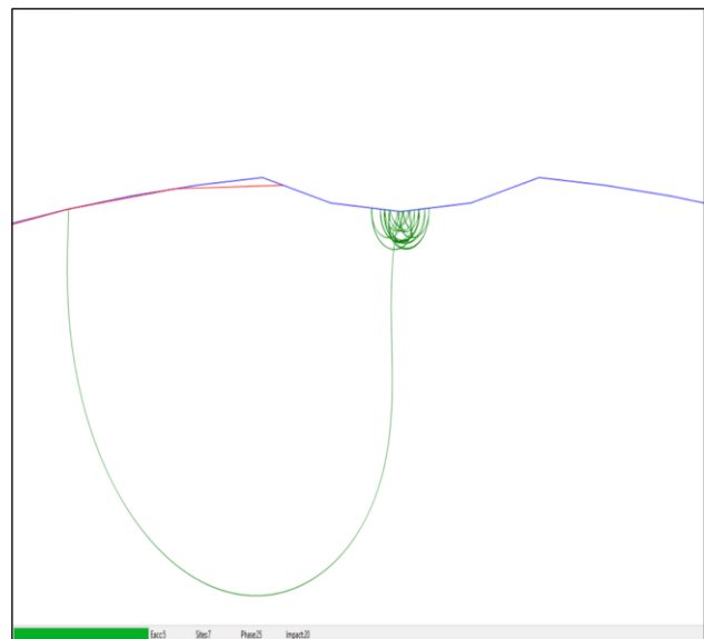
Figure 11: Electron trajectory in LB650 Cavity with Weld
