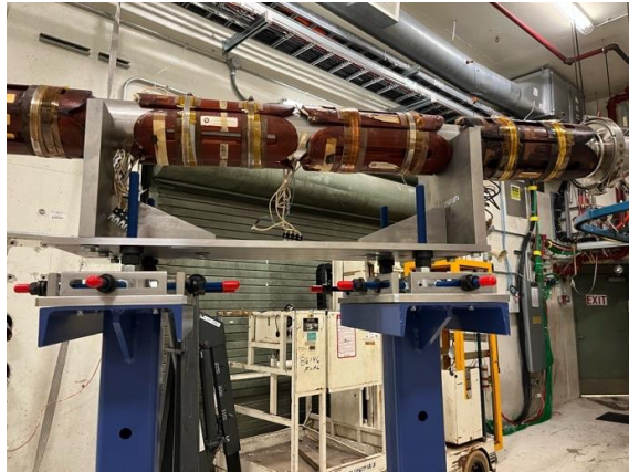
Figure 2 Picture of current air core quadrupole located in the MTA Hall.
