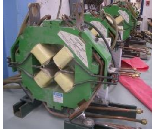
Figure 3 Future upgraded low carbon steel core quadrupoles.
