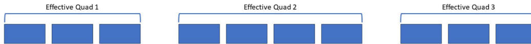
Figure 1 Current FODO cell configuration consisting of a matching quadrupole as the first cell, a focusing quadrupole for the second cell, and a defocusing quadrupole for the third cell.
