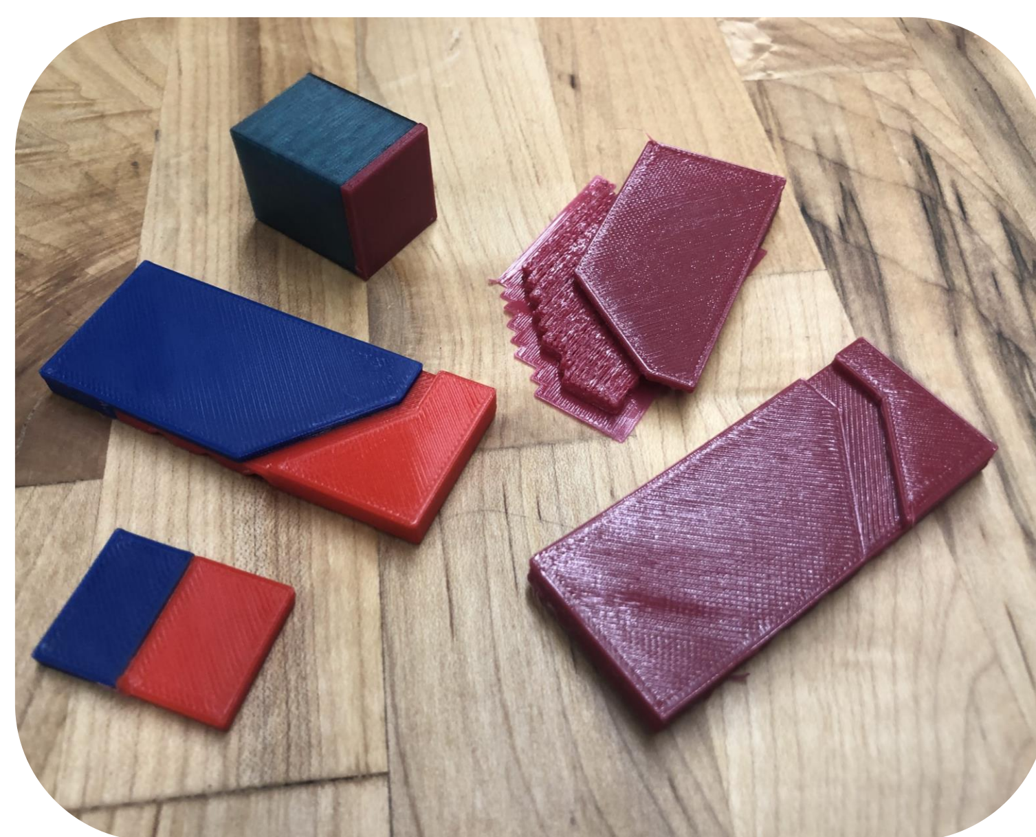
Test 3D prints experimented with various methods of combining different materials.
