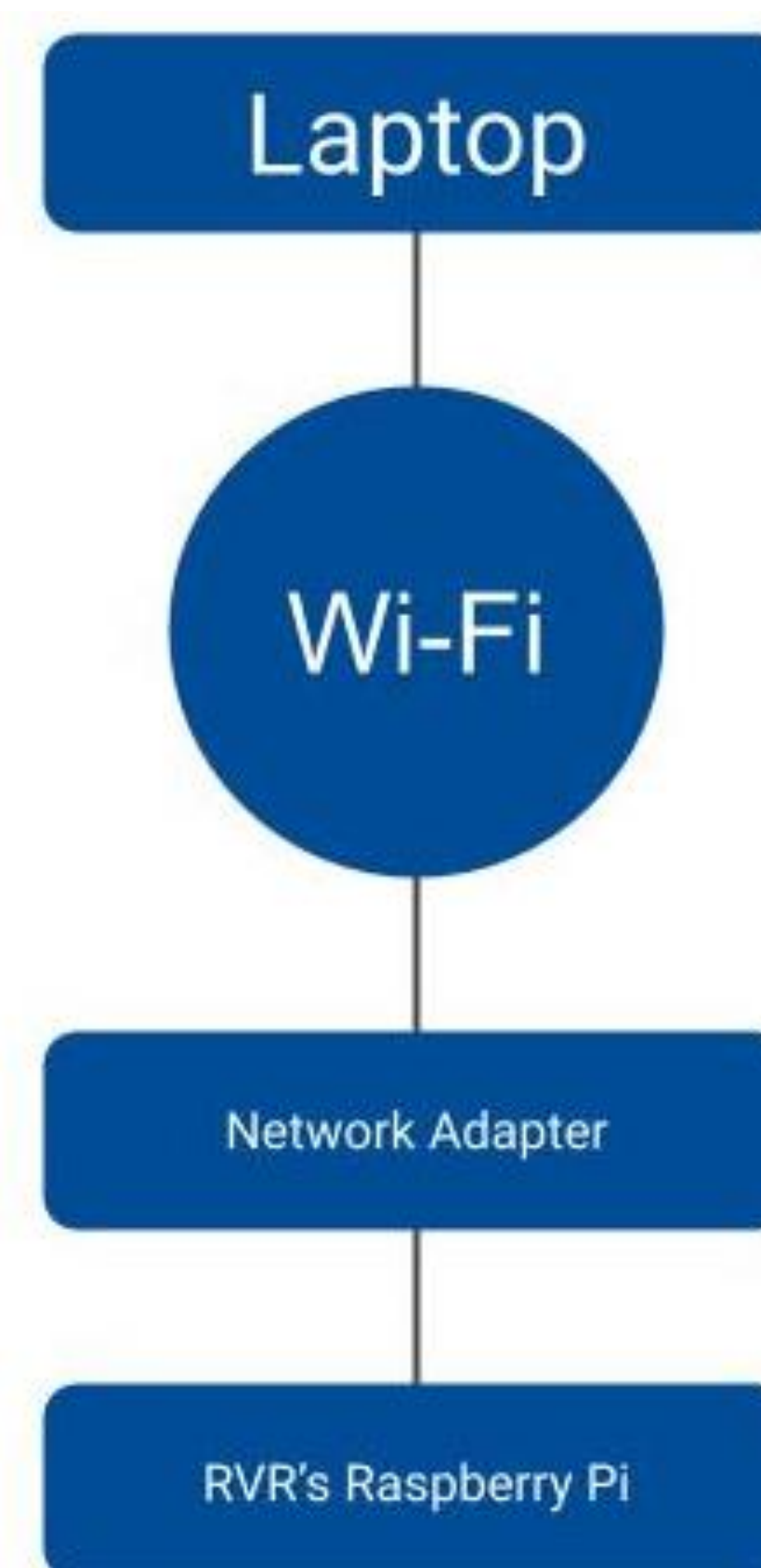
The new Raspberry Pi program runs motor commands sent from a laptop over Wi-Fi.
