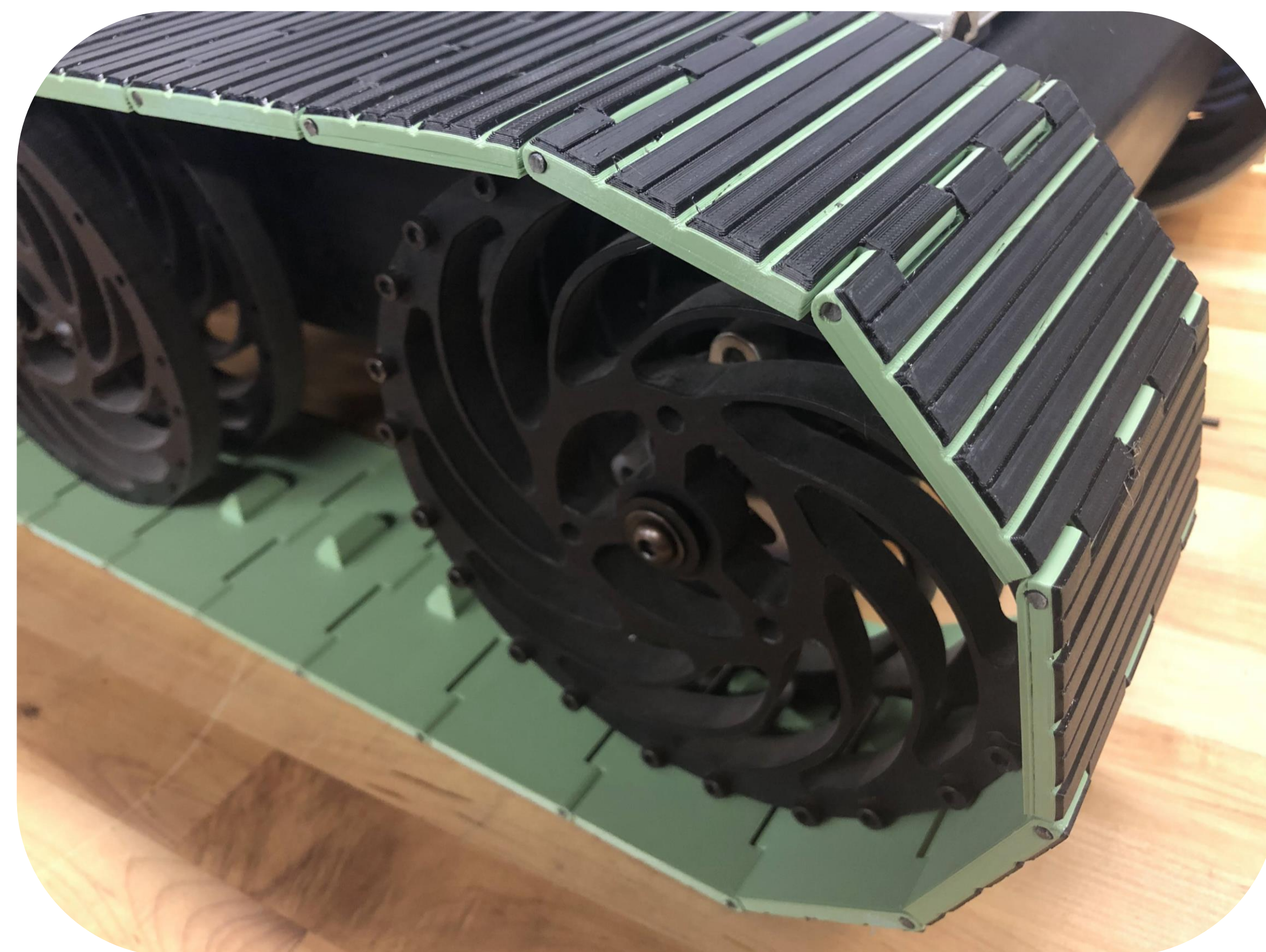
The track link's final design was printed out of two materials, TPU (black) on the bottom for traction and PETG (green) for structure and strength.
