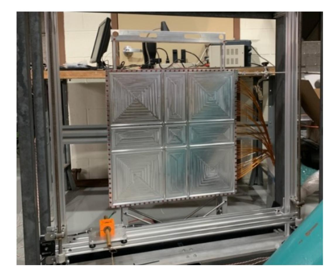
However, after reviewing the setup used to measure the sensor's output, we noticed that the metal plate used to reflect off the infrared light might've been unstable and shaky when recording data. This could be due to factors such as the plate being long and relatively thin, which could've resulted in small vibrations that went unnoticed.
