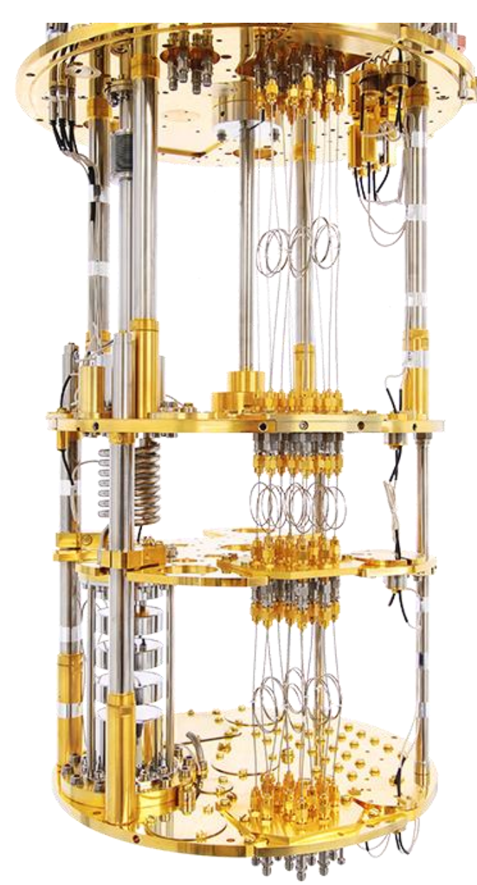
The inside of dilution refrigerator that provides continuous cooling to temperatures as low as 2 mK
