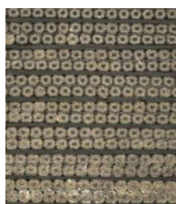
Image 1: Magnification of Nb 3 Sn ten stack layers comprised of a stainless-steel core, the conductor itself, reacted S 2 /Resin/Mica composite, and Pure Resin.
