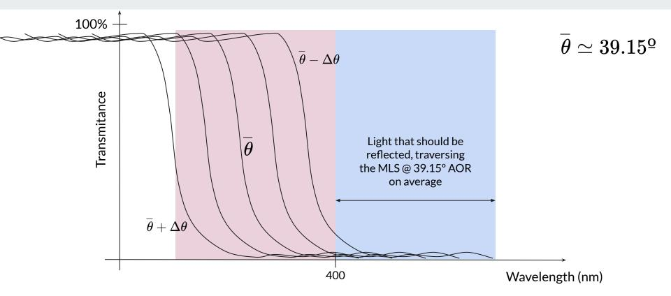
The angle distribution of this light within the MLS will have some spread  $\Delta \theta$  around the mean angle  $\theta$ . Ideally, all of the transmission curves within that angle spread should be **reflective** to the **WLSp light**.
