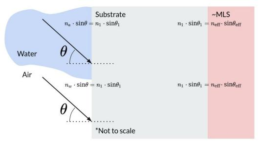
Within this model, to explain the dependence of TCs with the surrounding media, our current hypothesis is that what determines the TC is the angle of refraction (AOR) within the ~MLS.
