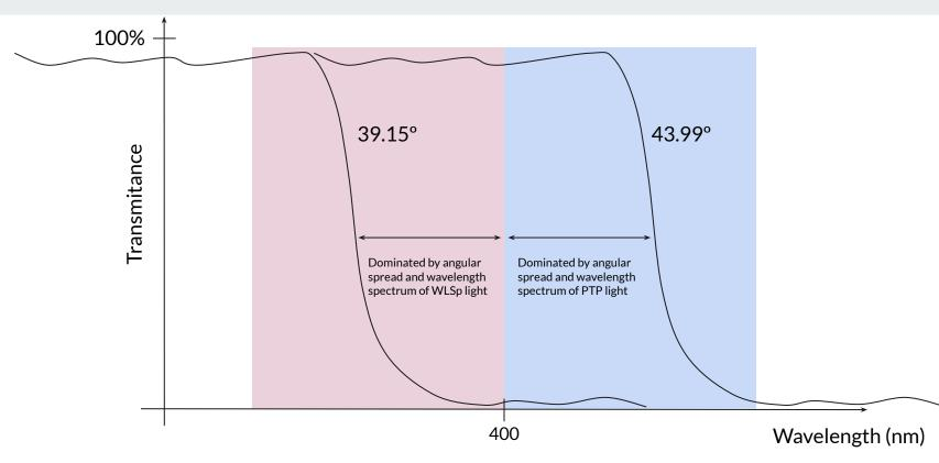
A first approximation taking into account both types of light should give an optimal cutoff at 400 nm at (39.15+43.99)/2 ° AOR in the MLS.
