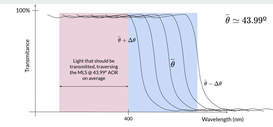
The angle distribution of this light within the MLS will have some spread  $\Delta \theta$  around the mean angle  $\theta$ . Ideally, all of the transmission curves within that angle spread should be **transparent** to the **PTP light**.
