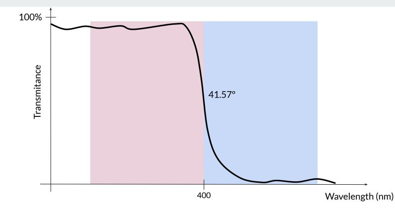
A first approximation taking into account both types of light should give an optimal cutoff at 400 nm at (39.15+43.99)/2 ° AOR in the MLS.
