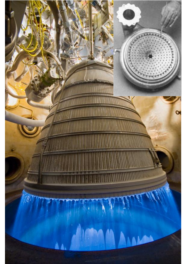
Aerojet Rocketdyne (L3 Harris) RL-10 Altitude Cell Hot Fire Test, Injector face inset
