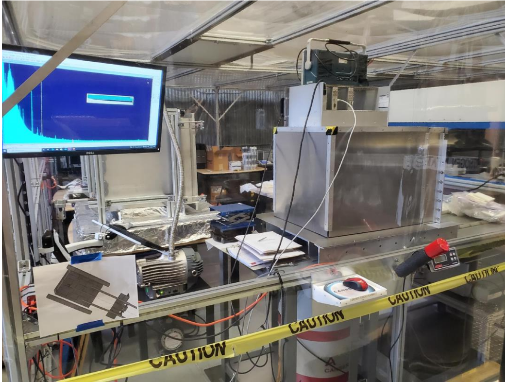
Physical setup of 'Rabbit' \gamma -ray BEGe detector
