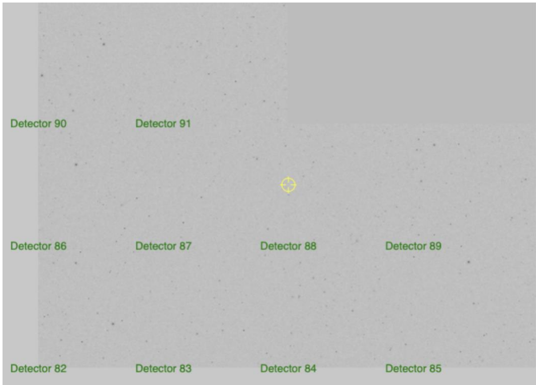
Figure 1. A mosaic view of detectors 82-91 using the mosaic notebook. (There are 189 detectors in the camera.) It is possible to zoom in to any of the individual detectors to view objects more closely.
