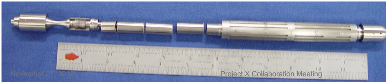
TMIST-2 In-Reactor Tritium Permeation Test Assembly with Real-Time Instrumentation and Control
