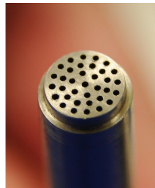
The holes shown in the end cap photo are 0.020 inches in diameter
