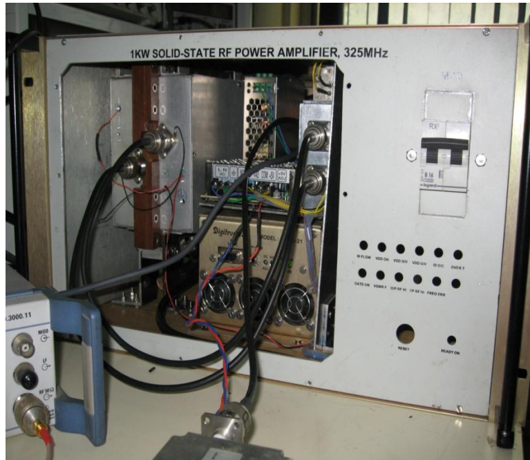
325 MHz, 1 kW unit under testing
