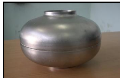
Prototype 1.3GHz cavity Nb half cells welded
