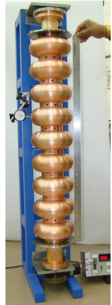
9-cell copper cavity
