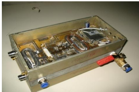
Two 1 kW RF units mounted back to back on heat sink
