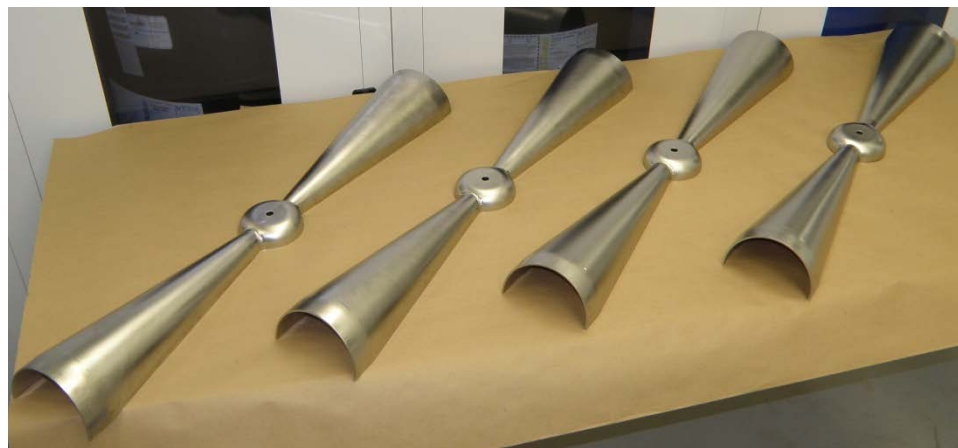
Center Conductors Ready For EDM
