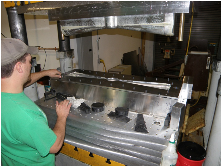
Center Conductor Pre-Forming
