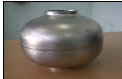
Prototype 1.3GHz cavity Nb half cells welded
