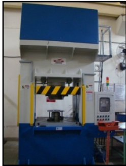
Cavity forming facility
