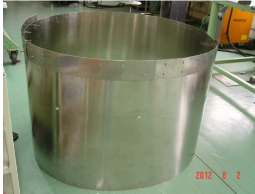
External Magnetic Shield segment under fabrication
