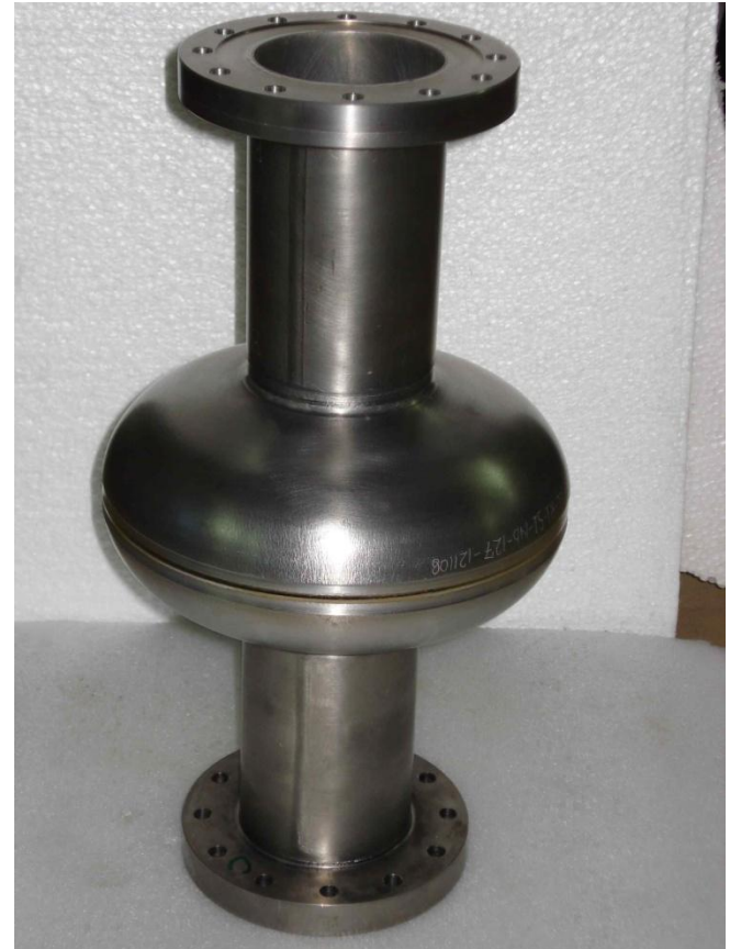
First 1.3 GHz Single Cell Niobium Cavity built in India
