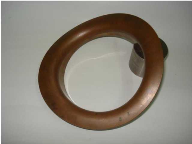
Spoke to Shell Collar (STSC) development using copper material
