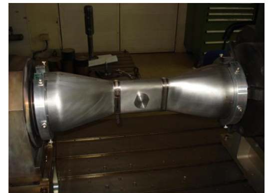
Spoke tacking setup
