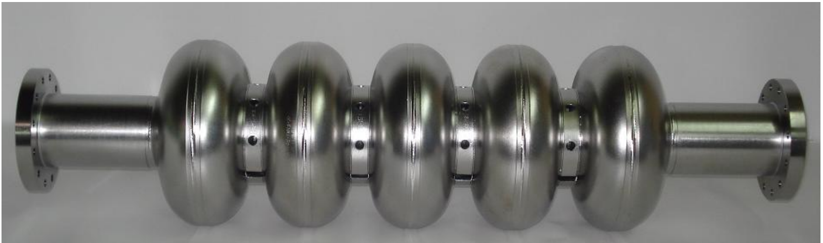
First 1.3 GHz 5-Cell Niobium Cavity built in India
