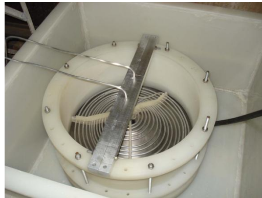
End Wall electropolishing setup
