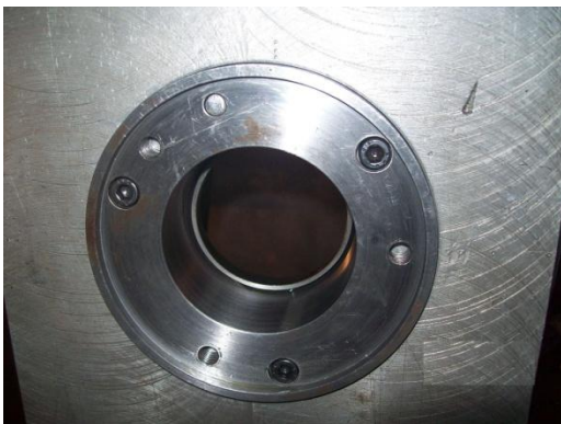
Coupler Port pullout in the Shell
