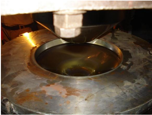
End Wall forming
