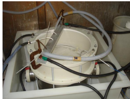
Outer Shell electropolishing setup
