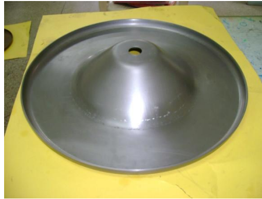
End Wall after forming
