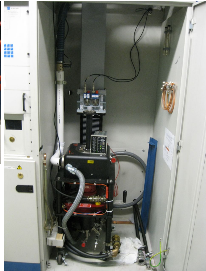
1.3 GHz 30 kW IOT @ MDB for horizontal test stand
